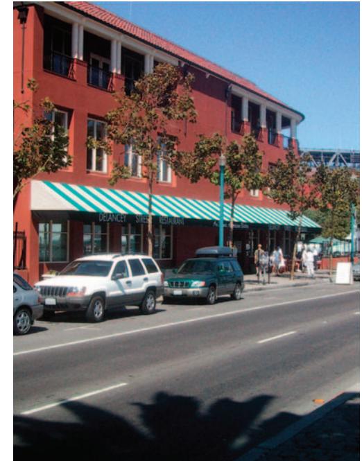
Large sweeping overhangs clearly separate the street level facade from upper facade.
